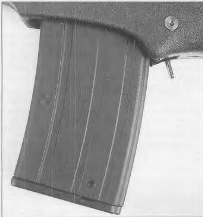
The magazine catch/release is directly in back of the magazine and similar to that of the R4. Like other Kalashnikov types, the magazine must be rocked forward for release from the magazine-well. A 20-round magazine is standard, but 35-, 30-, 25-, 15-, 10- and 5-round capacities are also available.
